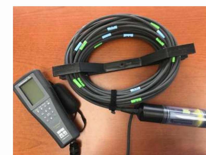
YSI Multi-Probe Measures water temp, dissolved oxygen, conductivity, and pH.
