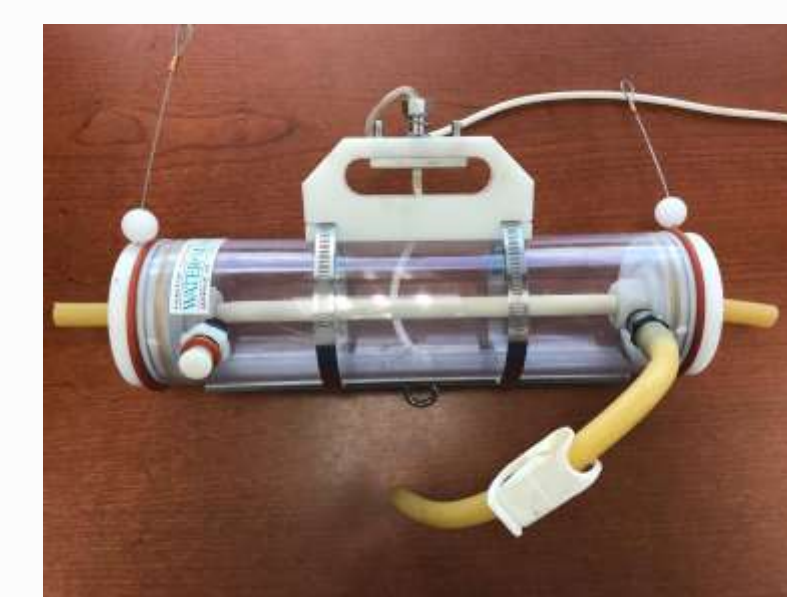
Van Dorn Sampler Collects water samples from specific depths within the lake.
