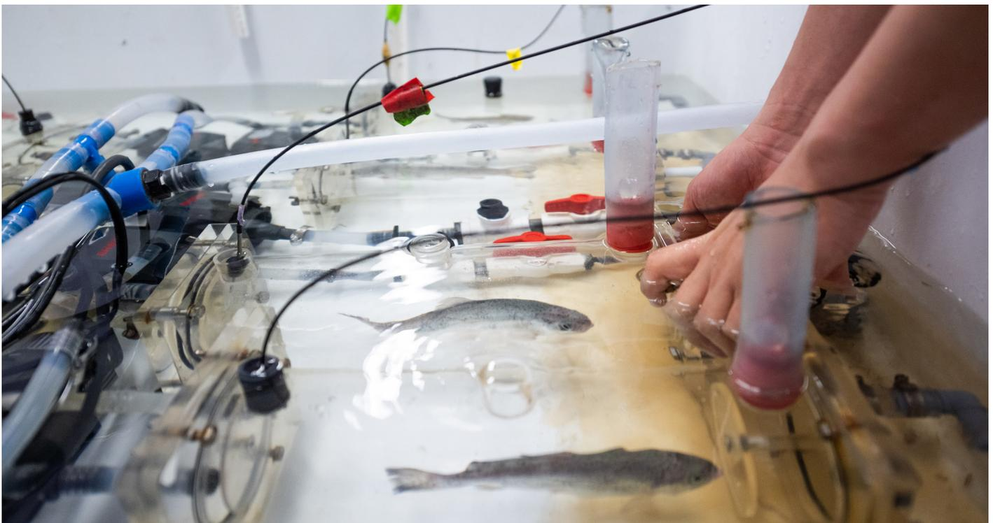
*Respirometers at the Hagerman Fish Culture Experiment Station designed to study oxygen consumption by redband trout.*
