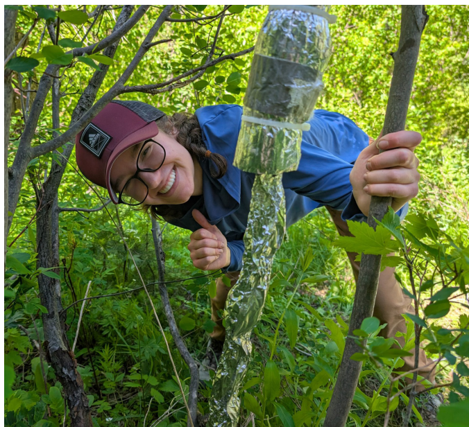
Hannah Bloxham, ISU SARE student, setting up a sapflow sensor to measure plant water use. Photo Credit: Sarah Godsey (ISU)
