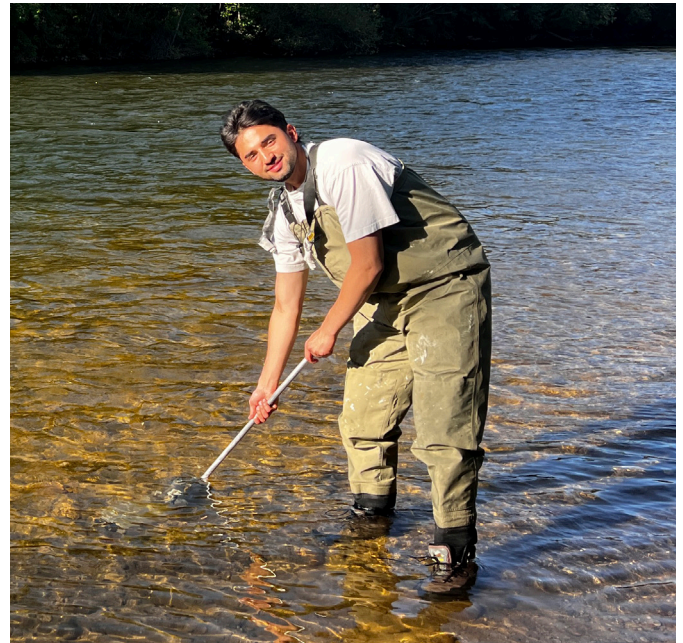
Ranjit Mainali, SARE student and Civil Engineering major at University of Idaho, collects sediment samples to characterize the bed grain size distribution and identify which particles are likely to be mobile under current flow conditions. Photo credit: Angel Monsalve Supulveda
