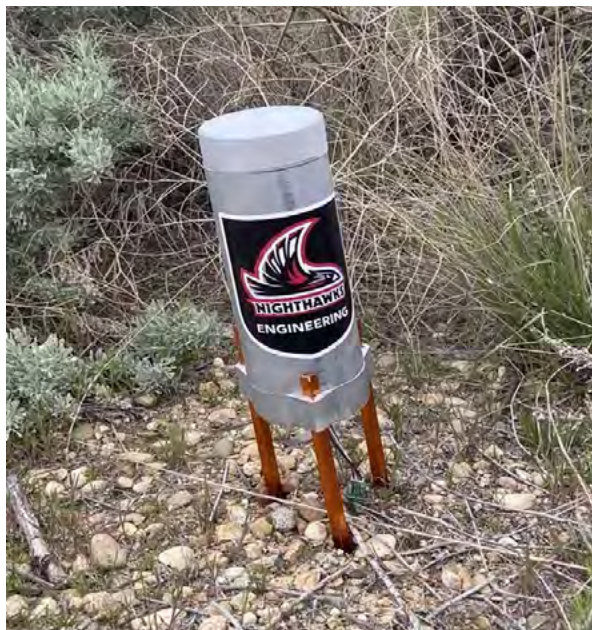
A prototype of the LIG sensor-tag created by the original team of NNU undergraduate students (Alex Nademann, Jonathan Ryan, Nick Irwin, Riley Mark, and Sam Mark) working on the project. The prototype electronics were housed in a plastic tube that could be mounted in close proximity to sagebrush.
