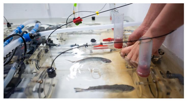
Respirometers at the Hagerman Fish Culture Experiment Station designed to study oxygen consumption by redband trout.
