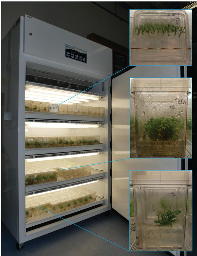
Growth chamber for propagating and maintaining the clonal lines of sagebrush for genomic and G×E research. The top inset shows how small cuttings of the clones are placed onto culture plates to allow for initial growth; the second and third insets show the clonal plantlets in boxes. These plantlets have grown roots and are developing biomass, which will be essential for getting enough leaf tissue for genome assembly. Photo credit: Peggy Martinez.
